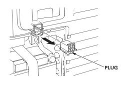
4. Pass the remote control cable through the battery maintenance co∨er knockout.
