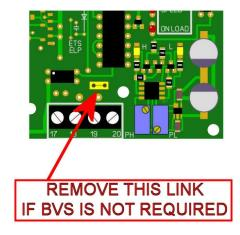
You may receive this configuration BVS link not fitted. Please fit it when required. Make sure your starting battery voltage is above 13.8V. Otherwise the generator may start immediately when link fitted.
