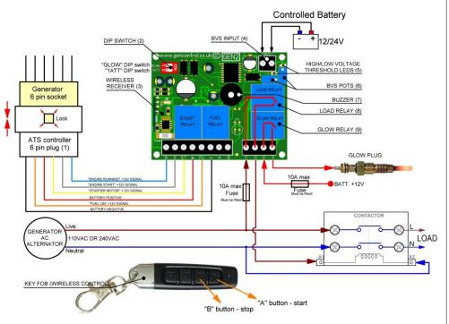
until the high voltage threshold detected (13.0Vdc set by default). These voltage thresholds are adjustable and can be set up by us precisely before shipment. Please let us know if you require any different BVS values.
