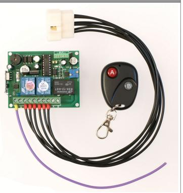
The engine run failure (low fuel shutdown or emergency stop) will trigger the continuous sound. This way the user will understand what happens to the generator not even looking at it. As an extra option the ATS controller may be supplied with the wireless key fob.
