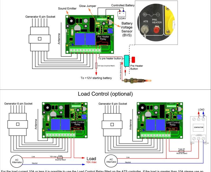
For the load current 10A or less it is possible to use the Load Control Relay fitted on the ATS controller. If the load is greater than 10A please use an appropriately rated contactor.
