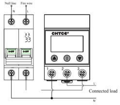
$\bullet$  Rated operating current of circuit breaker is 75% maximum current of voltage relay. I e = 0 . 7 5 I m a x
